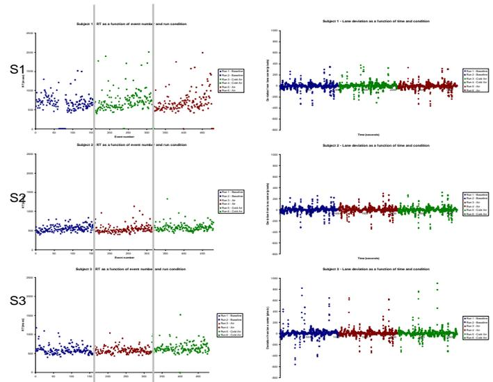
Figure 11. Reaction time performance of visual event detection (left panel) and standard deviations of lane tracking from the center of the lane during simulated driving (right panel) during simulated driving [blue color=baseline driving condition; green color=driving with cold air; red=driving with air].
