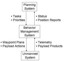
The BMS implements a set of activities or decision aids that accept plans and immediate taskings and turns them into actionable waypoint and payload inputs for unmanned systems. On the northbound interface, the BMS accepts telemetry and payload products and provides Situational Awareness and other systems access to the status of plans/tasks.
