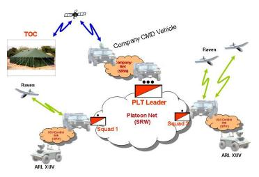
TC software resided at the Squad vehicle at Ft.Dix. Group commander software resided at the TOC (communicating over a SATCOM or SRW link) or Company command vehicle.
