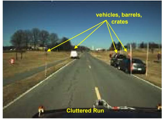
**Figure 5:** “Cluttered” configuration for Safe Operations experiment at NIST in January, 2009. Note vehicles, barrels, crates, and other objects not present in the “open” configuration.
