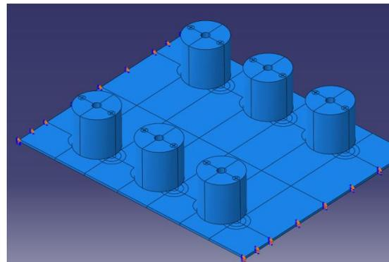
**Figure 2-a:** CAD model of PCB with large components
