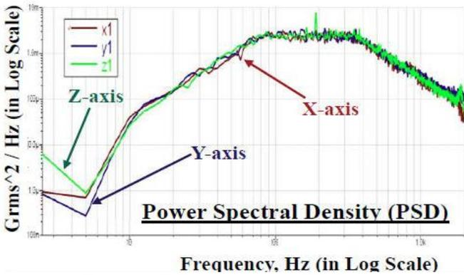
Figure 8: PSD in Multi-axial ED Shaker
