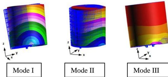
**Figure 11:** Inductor modal shapes when fixed at leads
