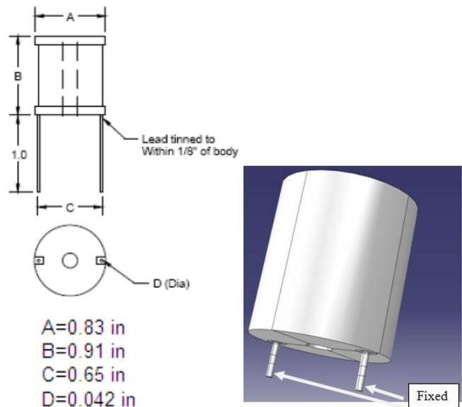
Figure 10: Large inductor used in this study
