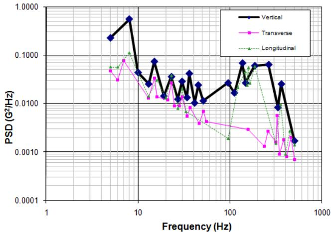
**Figure 3:** Composite two-wheeled trailer vibration profile
