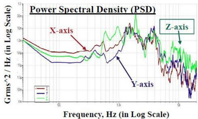
Figure 5: PSD in RS Shaker [18]
