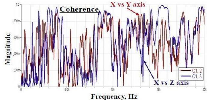
Figure 6: Coherence in RS Shaker [18]
