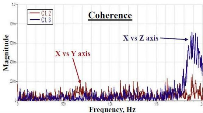
Figure 9: Coherence in Multi-axial ED Shaker
