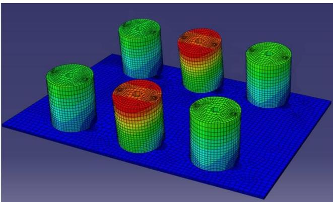
**Figure 12:** Middle Inductors first modal response in PCB
