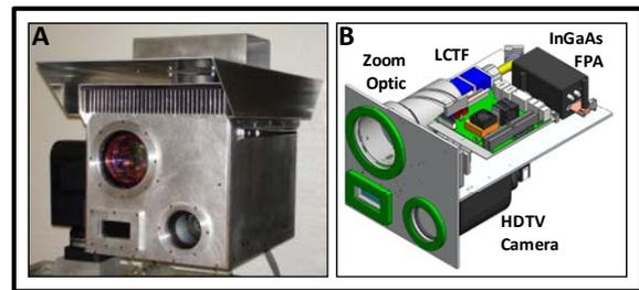
**Figure 1: (A) Digital Image of LightGuard Sensor (B) Diagram of LightGuard internal components.**
