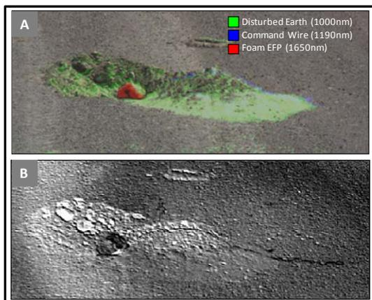
**Figure 2:** (A) The detection image of a scene containing disturbed earth, command wire and foam EFP. Disturbed earth detection is shown in green, the blue line shows the detection of command wire while the detection of foam EFP is shown by red; (B) The SWIR absorbance image extract collected from the scene.\*
