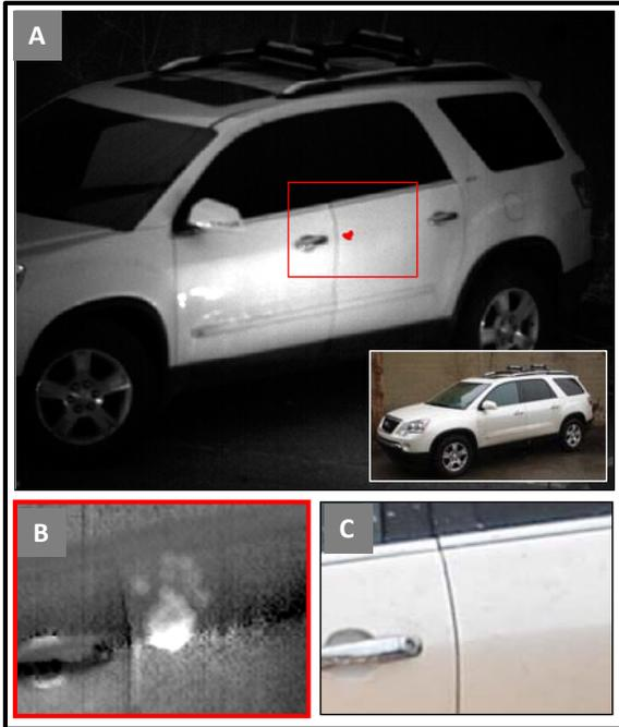
**Figure 5:** (A) shows the detection image of an AN handprint on a car door. The detection is characterized by the red marking; (B) shows the zoomed in absorbance image of the AN handprint; and (C) shows a digital image of the car door where the handprint is located.
