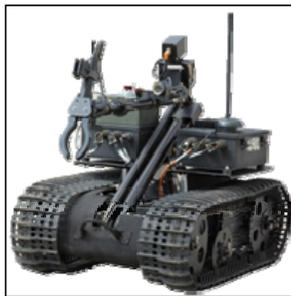
**Figure 9:** Conceptual design showing the STARR sensor mounted to the TALON robot.
