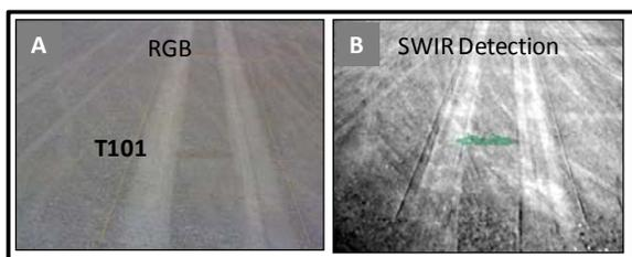
**Figure 3:** (A) Digital image of target 101; (B) Detection image of target 101. The green marking indicates the location of disturbed earth.\*
