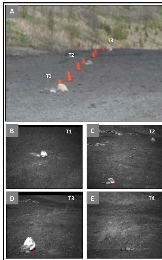
**Figure 4:** (A) Digital Image showing the location of AN targets; (B-E) Detection images associated with the AN targets. The red markings indicate an AN detection.
