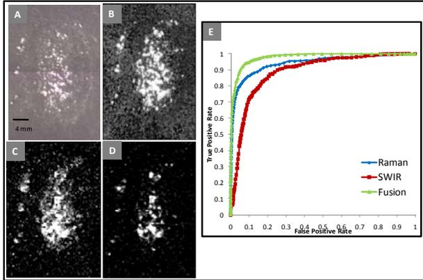
**Figure 8:** Example of Sensor Gain improvement. (A) shows the RGB image of the AN fingerprint; (B) shows the 1570 nm SWIR image; (C) shows the fusion image; (D) shows the 1040  $\text{cm}^{-1}$  Raman image; and (E) shows the ROC curves associated with the Raman  $P_D$  (blue), SWIR  $P_D$  (red) and the fusion  $P_D$  (green).
