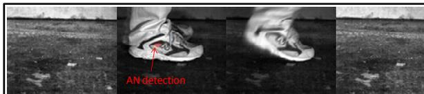
*Figure 7: AN detection on a person's shoe, moving through the scene.*
