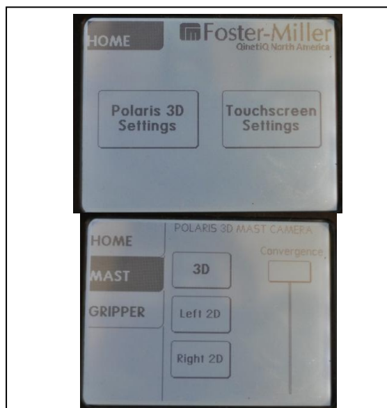
Figure 6. Touchscreen interface used to adjust 3D stereo convergence on the mast camera and other 3D settings.
