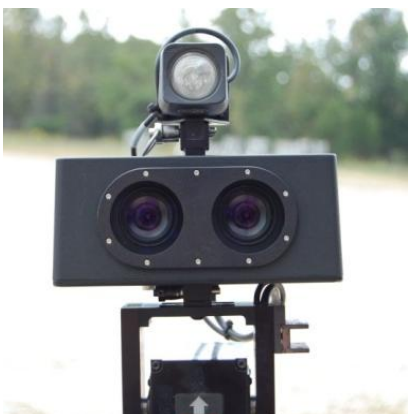
Figure 5. The stereo mast camera mounted on pan / tilt stage with illuminator.
