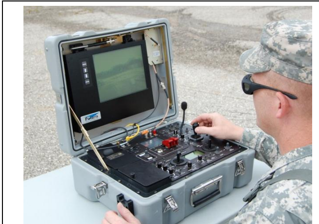
Figure 3. Soldier using the TALON operator control unit equipped with the Polaris 3D upgrade kit. The operator is wearing polarized glasses. Note that the display is daylight readable, and does not require the shroud used in 2008.
