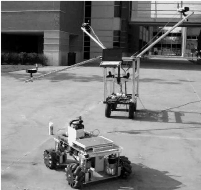
Fig. 2: UWB base station test rig and Mecanum ODV
