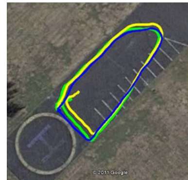
Figure 5: Loop closure test: Yellow – GPS, Green – GPR + RF; Blue – Visual Odometry.
