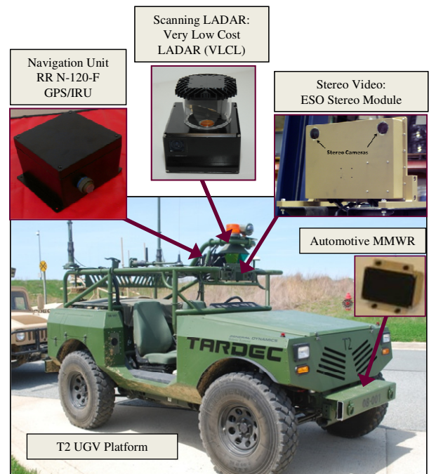
Figure 2 - SOURCE Low Cost Sensor Suite Configuration for Capstone Experiment
