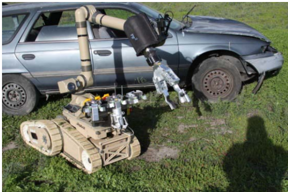
Figure 2. Warrior platform outfitted with gripper showing "toolbelt" to carry additional end effectors
