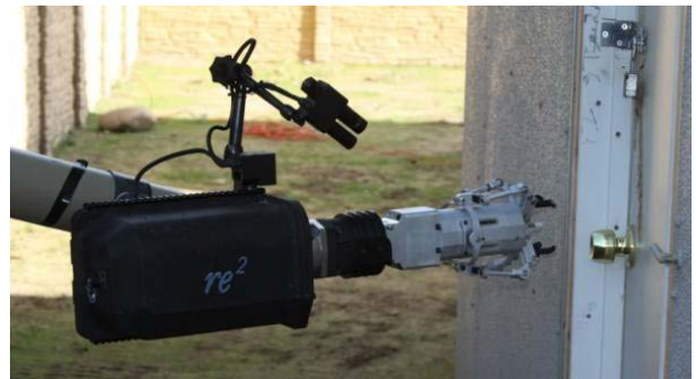
Figure 1. Warrior tool change technology outfitted with TARDEC-developed door opening end effector
