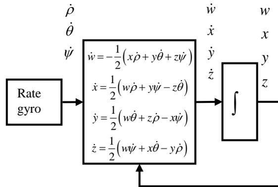
Figure 14: Quaternion kinematics model
