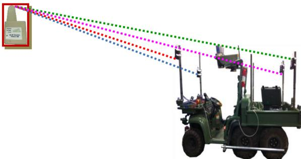
**Figure 8:** Mobile UWB LPS in a radiating configuration for tracking objects.
