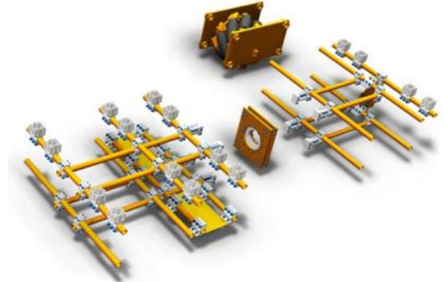
**Figure 3:** Flexible space frame construction conveniently allows resize and reshape of an AGV platform.
