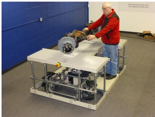
Figure 5: OmnicO AGV with payload and walk-on work platform.
