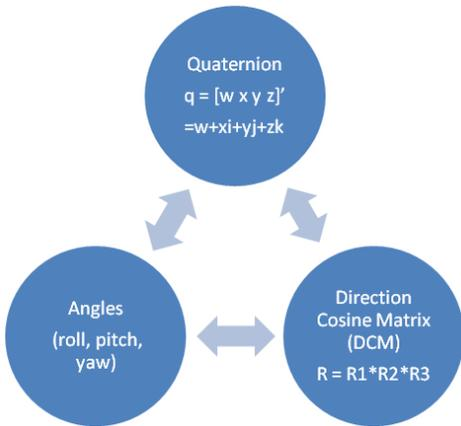
Figure 13: 3D kinematic transformations
