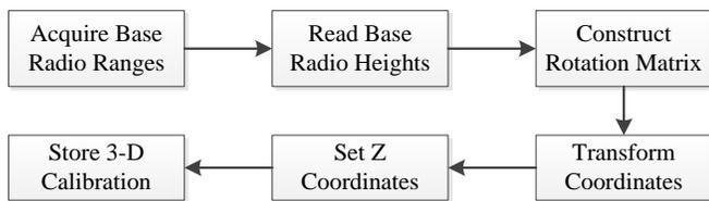
**Figure 10:** UWB calibration procedure.
