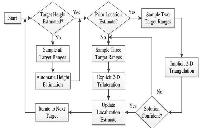
**Figure 11:** Flowchart of the localization algorithm
