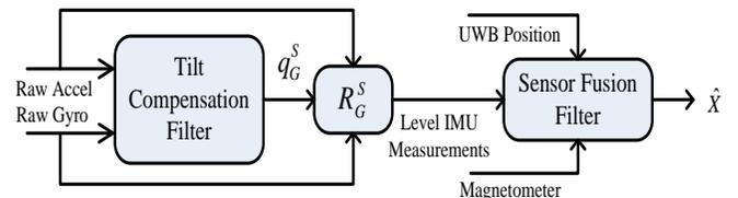
**Figure 12:** Navigation estimation/filtering approach.
