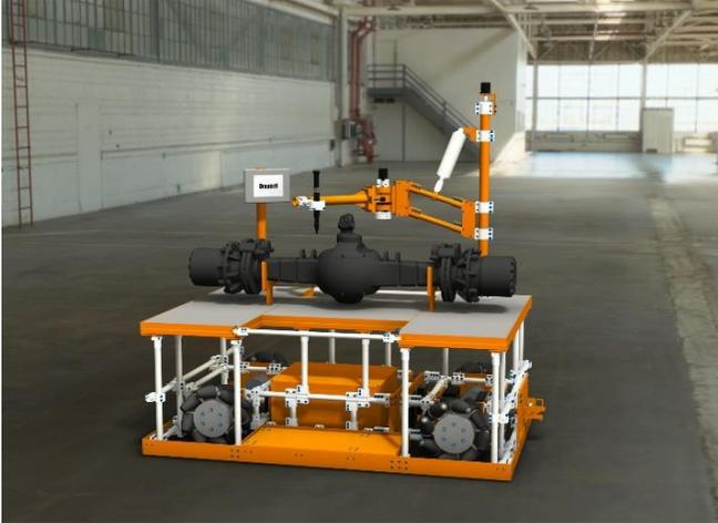
**Figure 1:** An OmnicO AGV developed for flexible and agile operation
