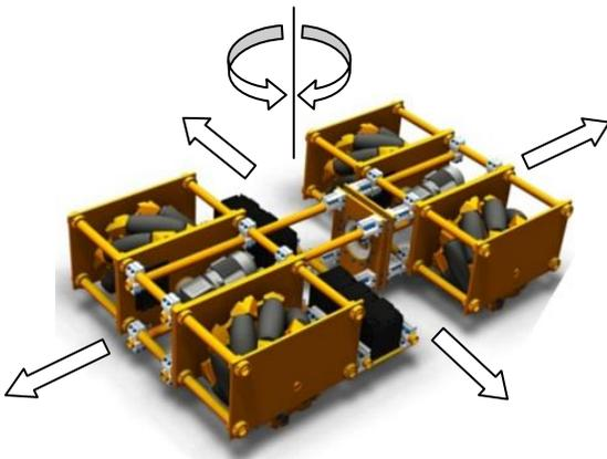
**Figure 2:** An omnidirectional AGV fitted with Mecanum wheel is able to move independently in different directions to provides agile mobility for speedy maneuvers.
