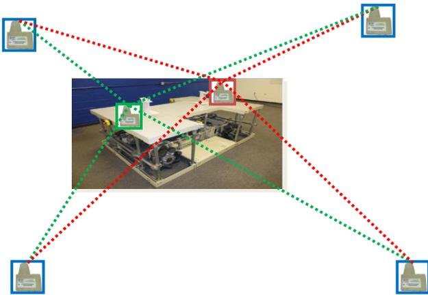
**Figure 6:** UWB LPS in a constellation configuration for accurate positioning.
