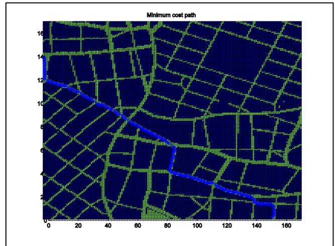
**Figure 11.** A random path through the AOI. By applying the route planner retrospectively, this path is shown to be sub-optimal for a UGV dependant on GPS data.
