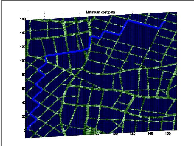
**Figure 9.** The route chosen when allowing for high GPS error when IMU error is low. This route successfully avoids the large area of GPS dropout near the bottom right corner of the AOI.
