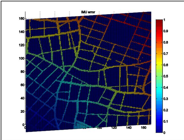
**Figure 6.** The predicted IMU sensor error along the road network.
