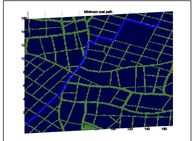
**Figure 8.** The route with minimum cumulative sensor errors.
