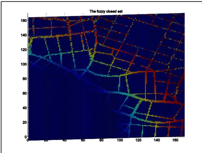
**Figure 10.** The road network with node costs for a UGV that requires either highly accurate LIDAR or highly accurate IMU/GPS data. Red nodes have a cost of -1 and are closed, and no route exists between the start and goal points in this case.
