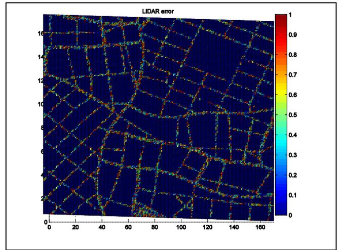
**Figure 5.** The predicted LIDAR error along the road network.
