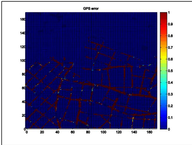
**Figure 4.** The predicted GPS error along the road network.
