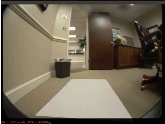
Figure 3: Example of predictive display using monocular imagery. The camera point of view is rotated to track the robot, transforming the image appropriately, and the predicted robot location is drawn in the image using a flat earth model and the trajectory implied by the sequence of commands input by the operator.
