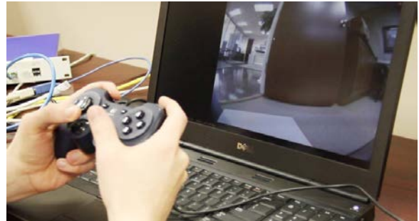
Figure 2: TORIS OCU interface. The OCU display shows the operator a latency-corrected predicted view of the robot’s relationship to the environment, and the user inputs commands representing desired travel distance and robot orientation using a standard game controller. Predictive display to compensate for system latency
