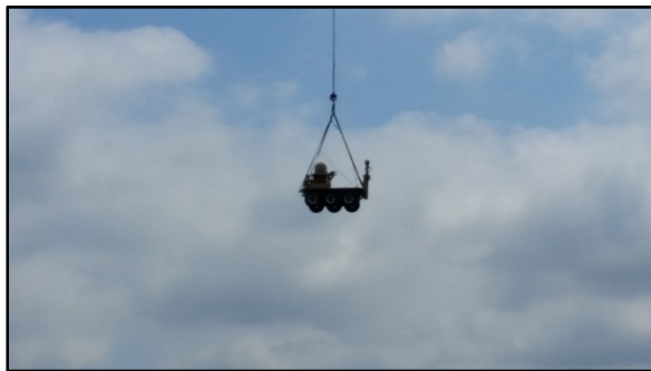
Figure 7: Close-up of SMSS in flight showing rigging system.
