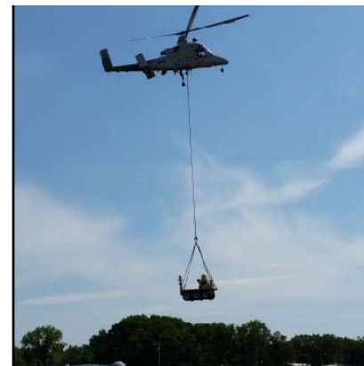
Figure 5: SMSS fully slung in lift by K-MAX.
