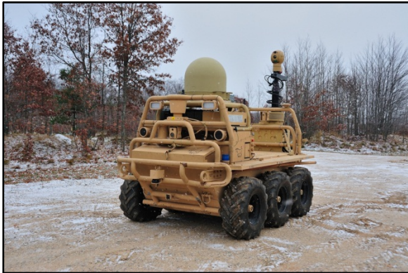
Figure 1: SMSS at Camp Grayling with General Dynamics SATCOM Technologies (GDST) SOTM unit mounted near the front top of vehicle and mast-mounted Gyrocam 9M on the rear of vehicle.
