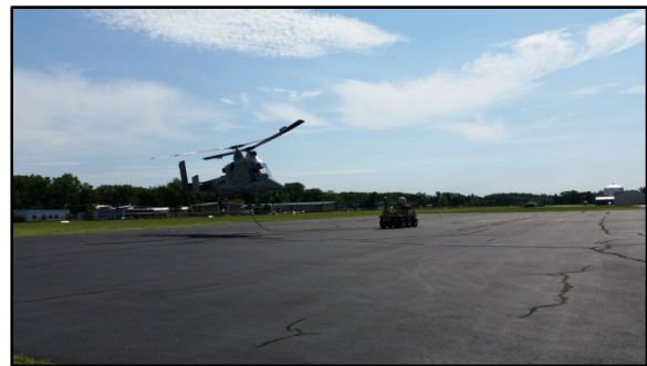
Figure 4: K-MAX starting lift with SMSS in sling rigging.
