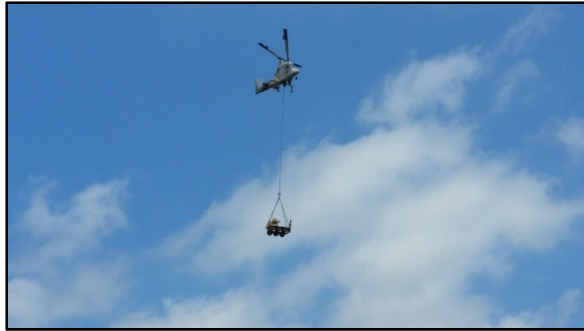
Figure 6: SMSS in flight under K-MAX at 50 kts showing stable aerodynamics.
