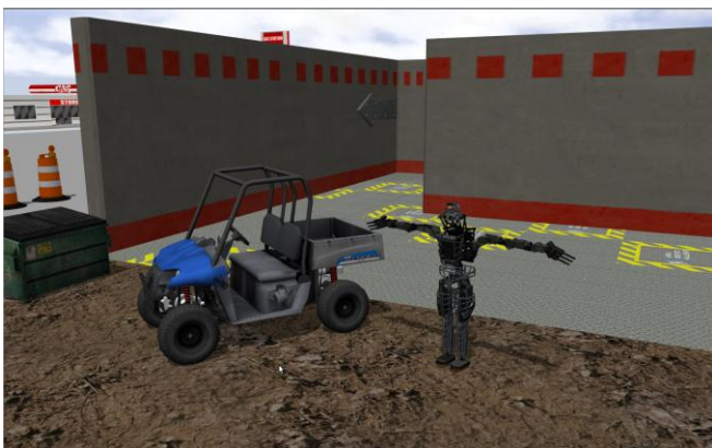
Figure 7: Example of Gazebo rendering of DRC robotic Atlas humanoid system, control vehicle and other terrain features
