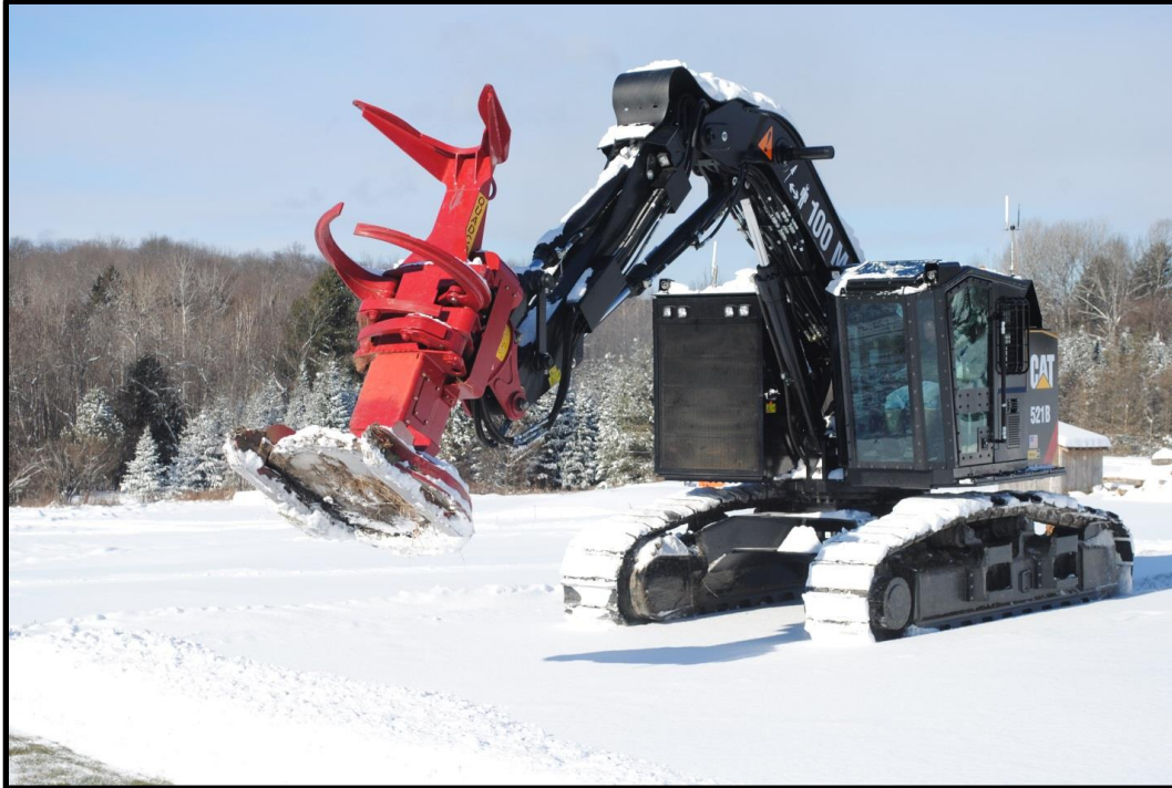
Figure 4. The antenna on the top right of the vehicle cab was mounted on a floppy spring, allowing direct hits from trees to easily deflect the antenna boom without causing antenna or cable damage.
