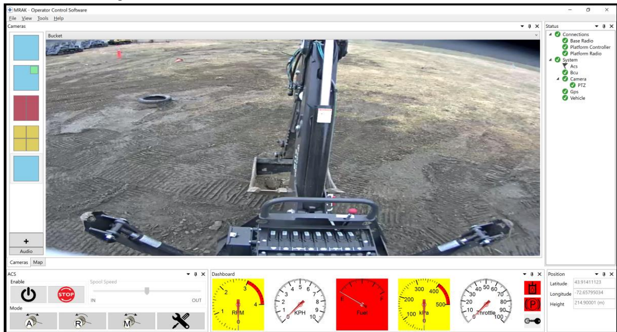
Figure 3. The User Interface for all M-RAK applied vehicles is largely the same, minimizing training time.
