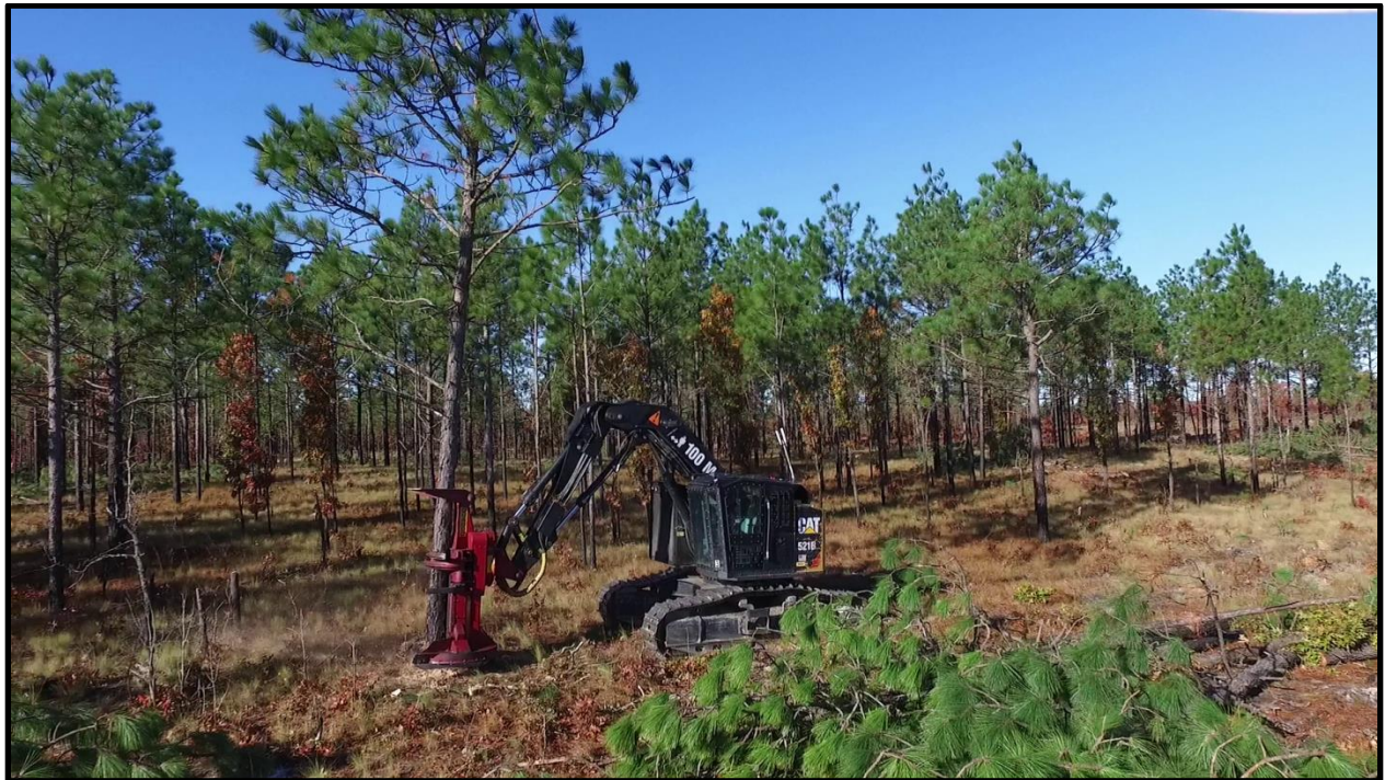
Figure 2. M-RAK controlled CAT 521b Tracked Feller Buncher clearing pine trees on a heavy artillery / helicopter range at Ft. Bragg, NC.
