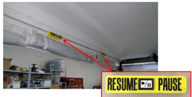
Figure 4. Pause/Resume buttons are located throughout the vehicle
