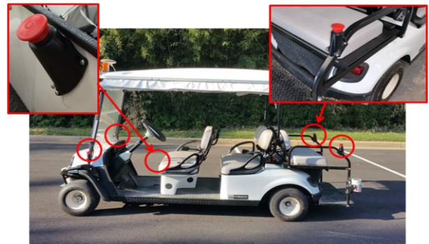
Figure 3. E-Stop system locations for safety operator and riders.
