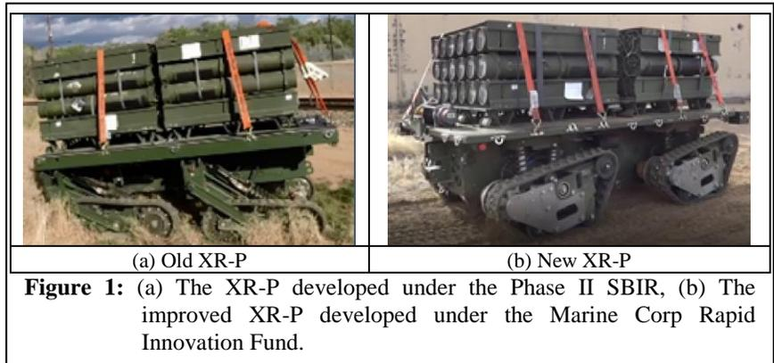
**Figure 1:** (a) The XR-P developed under the Phase II SBIR, (b) The improved XR-P developed under the Marine Corp Rapid Innovation Fund.
