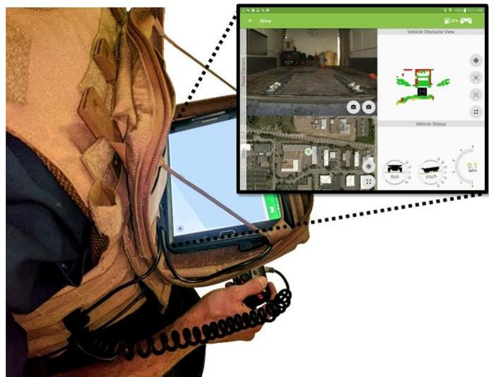
**Figure 9:** The Android based Operator Control Unit. A joystick is connected to the tablet for Assisted-Teleoperation. The operator wears a small backpack that contains the wireless radio and batteries.
