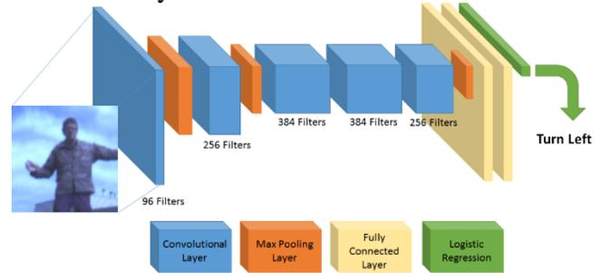
Figure 6: The architecture of our AlexNet based CNN.
