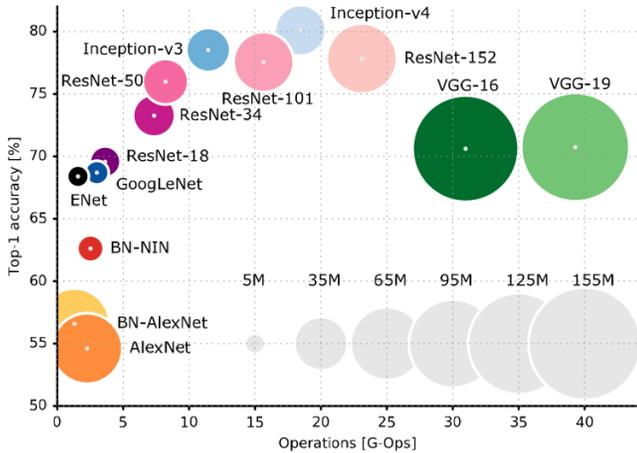
Figure 5: Comparison of popular CNN architectures. The vertical axis shows top 1 accuracy on ImageNet classification. The horizontal axis shows the number of operations needed to classify an image. Circle size is proportional to the number of parameters in the network.
