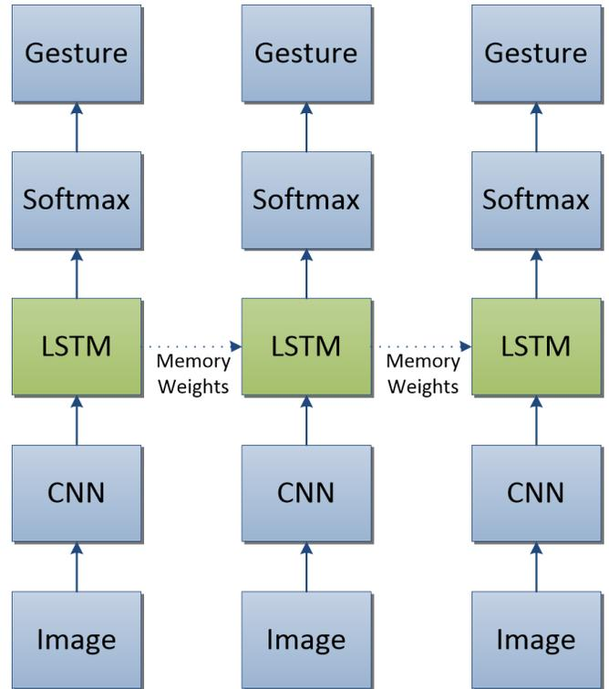
Figure 8: Gesture recognition architecture with the addition of a LSTM between the CNN and the softmax layer.
