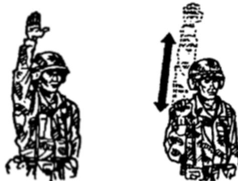
Figure 3: Halt (left) and Increase Speed (right).
