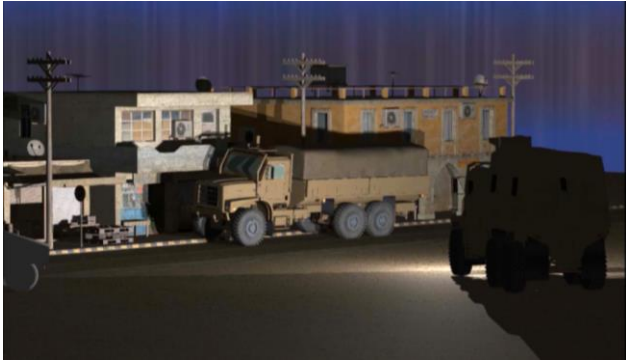
Figure 11: Example real-time ray traced image using the software, including shadows and texturing for terrain and truck surfaces. Shadowing and reflection are emergent behaviors.
