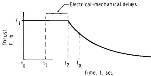
Figure 13 Rocket thrust engine characteristics [15]
