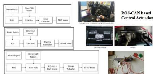
Figure 2. Oakland University’s Self-Drive Vehicle Control Diagram.
