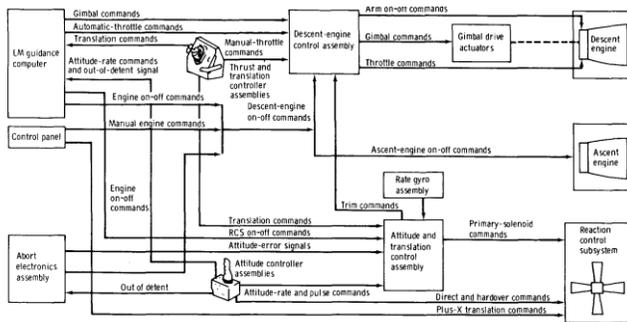
Figure 14. block diagram of the SCS[16]
