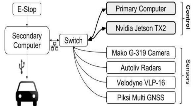
Figure 4. Lawrence Technological University's Self-Drive vehicle safety/processing/sensor overview schematic.
