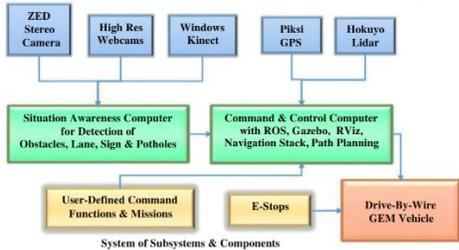
Figure 3. Oakland University's Self-Drive Vehicle Sensor Functions Diagram.
