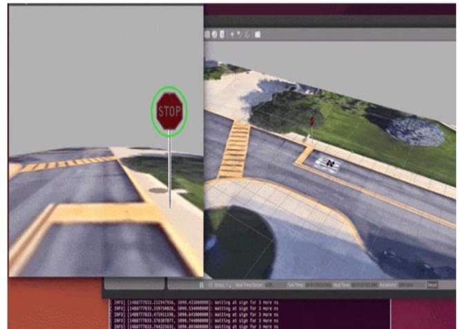
Figure 9. LTU Self-Drive vehicle simulation testing with relevant simulated environment (road signs, lane markings, etc.)<sup>7</sup>
