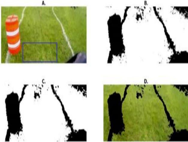
Figure 5. Stony Brook University vehicle camera extracted histogram projection.<sup>1</sup>
