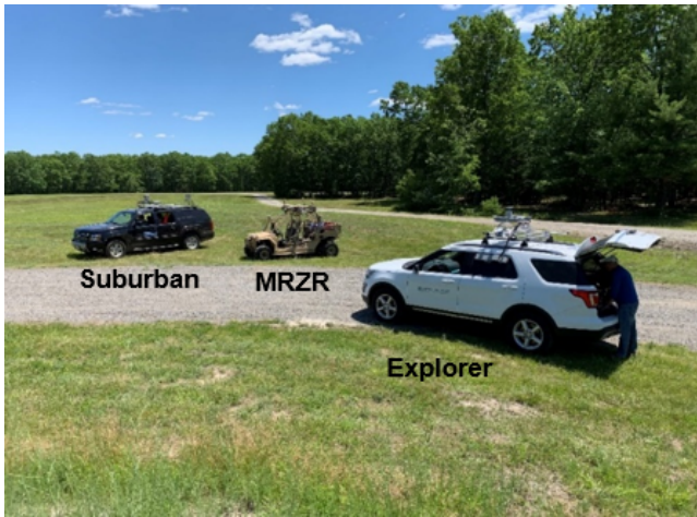
Figure 12: Vehicles used for our data collection at Fort Devens. The MRZR and Suburban were target vehicles, while the Explorer equipped with the DCK was the observer vehicle.
