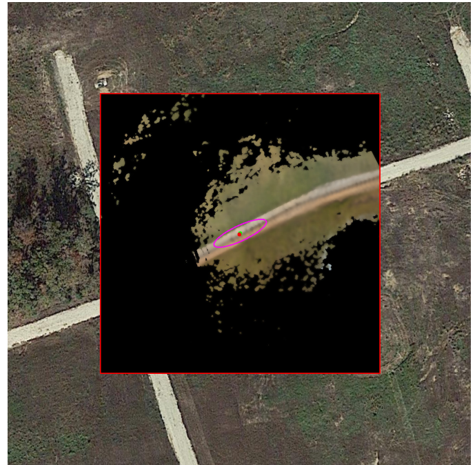
Figure 2: The template image T overlaid on the satellite source patch image \bar{S} at the match location. The red dot represents the UGV's location prior while the green dot shows the ATLIS proposed update. The pink ellipse displays the 95% confidence interval for the estimated covariance matrix.
