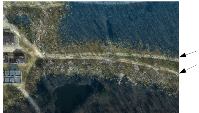
Figure 15: Road Diverges as Error Compounds without Loop Closures in RTABMap using GraphSLAM
