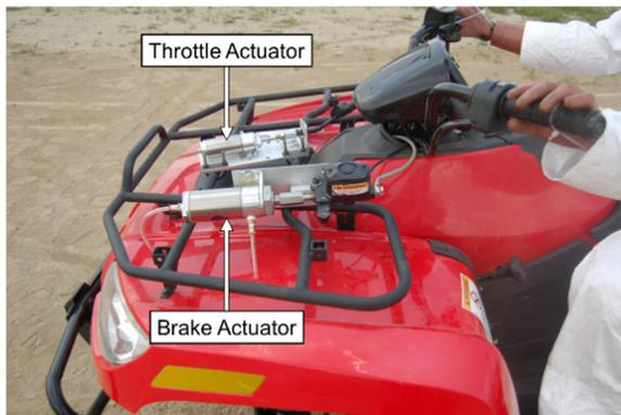
Figure 10: ATV Throttle and Brake Actuators
