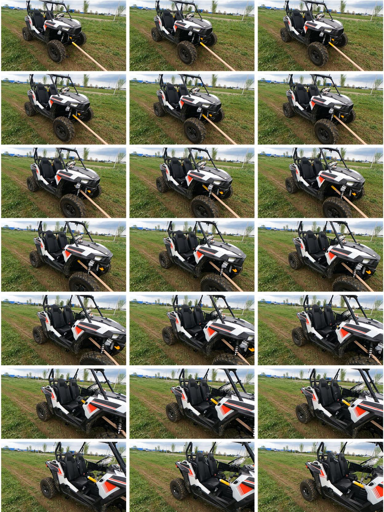
Figure 7: Time Lapse Images of ROV Zone 1 Penetration
