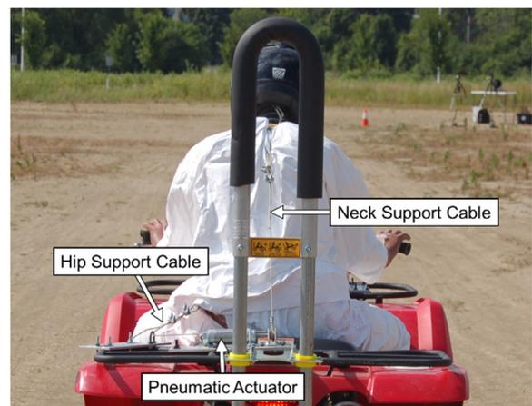
Figure 11: Secure-and-Release System Cables
