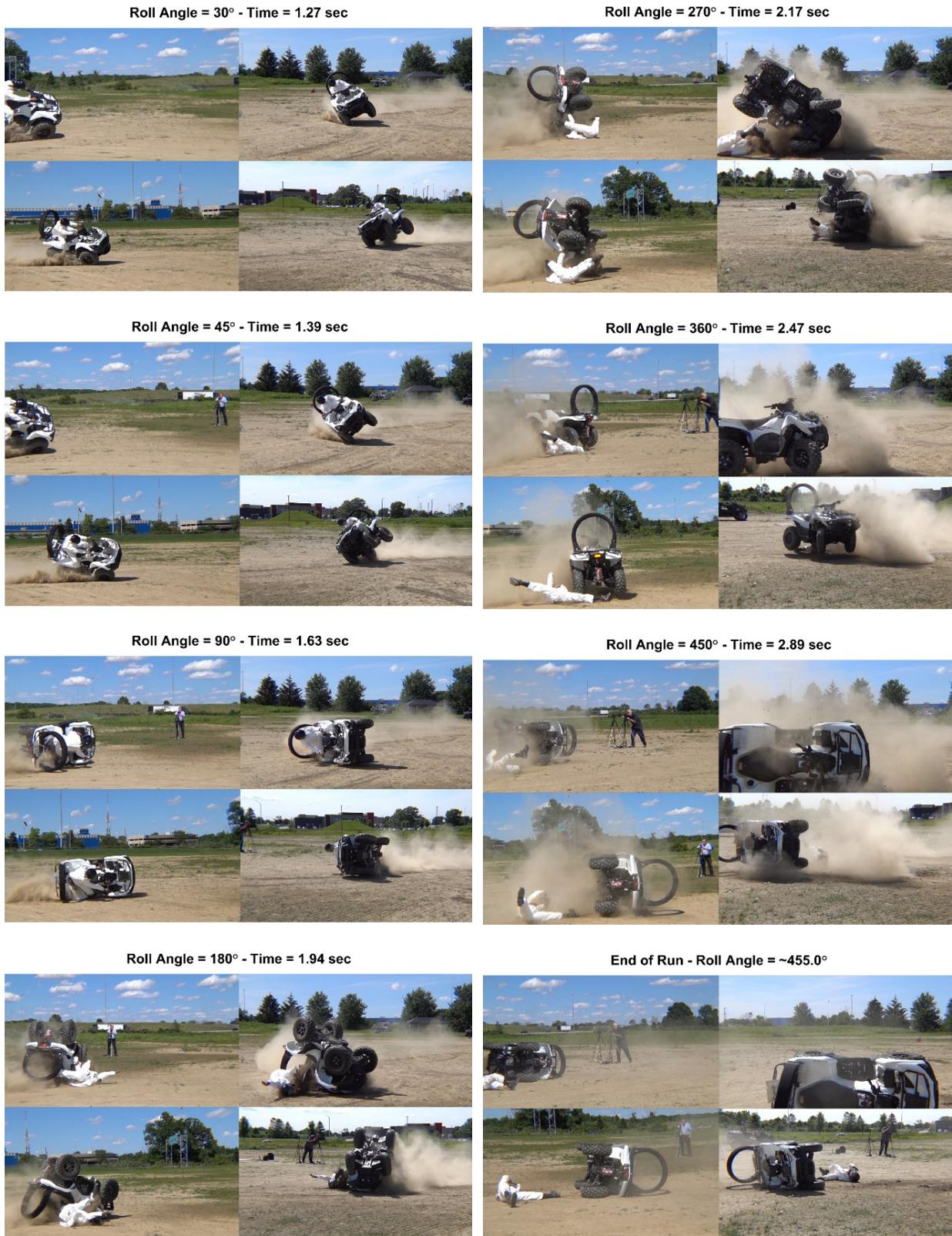
Figure 12: Rollover Sequence Images from a Moderate Energy Rollover Event
