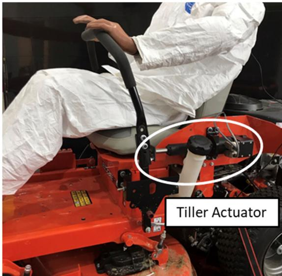
Figure 13: ZTM ATD Tiller Actuator
