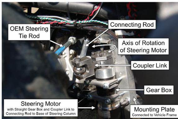
Figure 9: ATV ATD Steering Actuator
