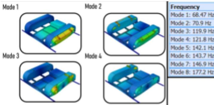
Figure 17: Vibration Modes with Constrained Corners
