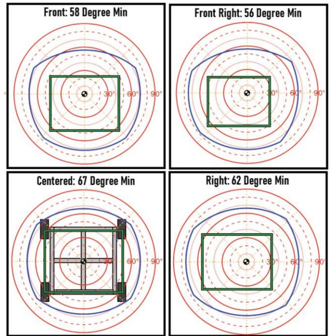
Figure 19: Tipover Stability (5in Center of Mass Height)
