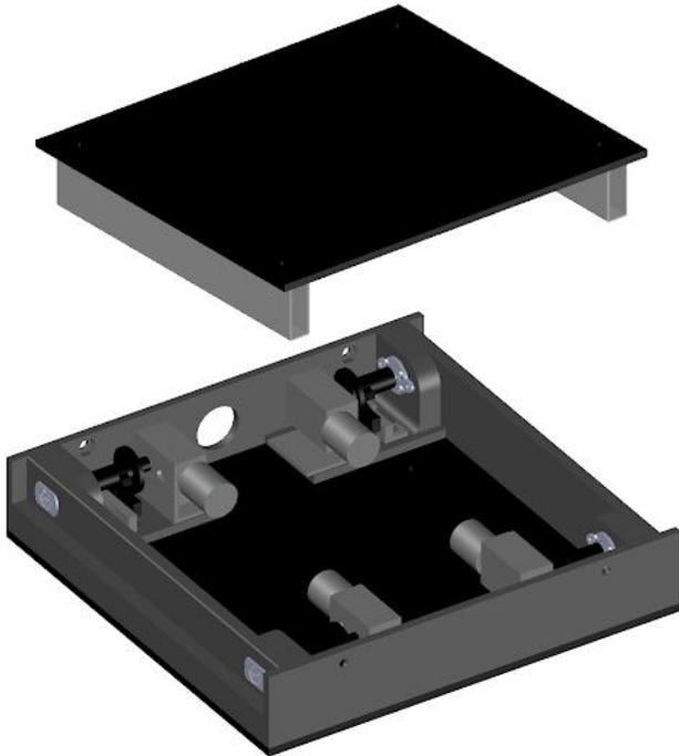
**Figure 23:** Modular Mounting Interface
