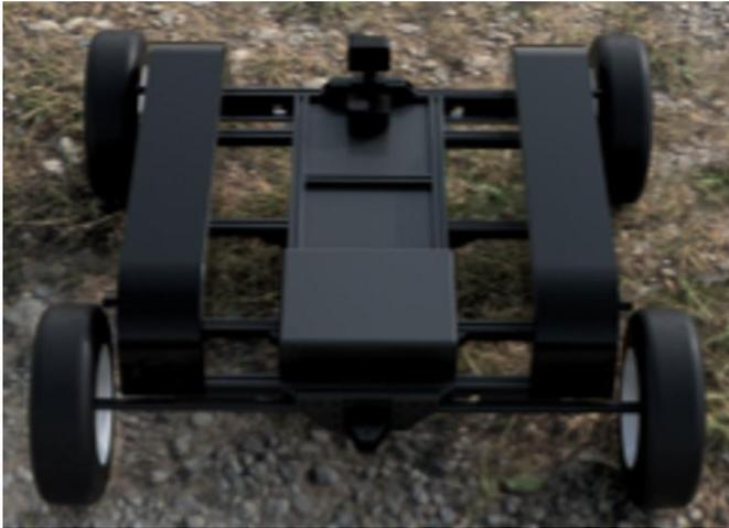
**Figure 14:** Modular Assembly UGV
