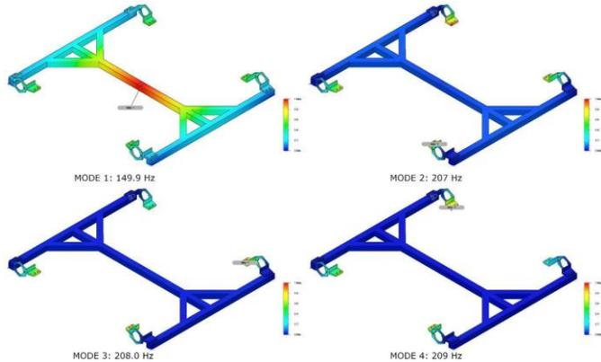
**Figure 12:** Lowest Frequency Vibration Modes
