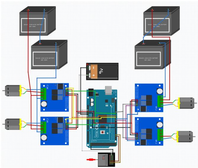
**Figure 15:** Electronic / Power Architecture
