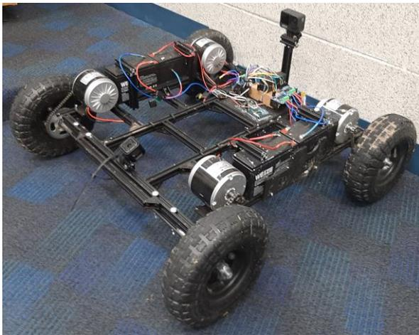
**Figure 21:** Modular UGV Prototype
