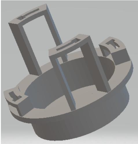
**Figure 8:** Payload Support Adapter
