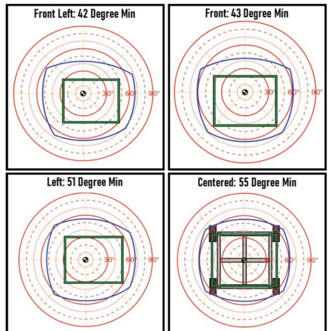
Figure 20: Tipover Stability (8in Center of Mass Height)
