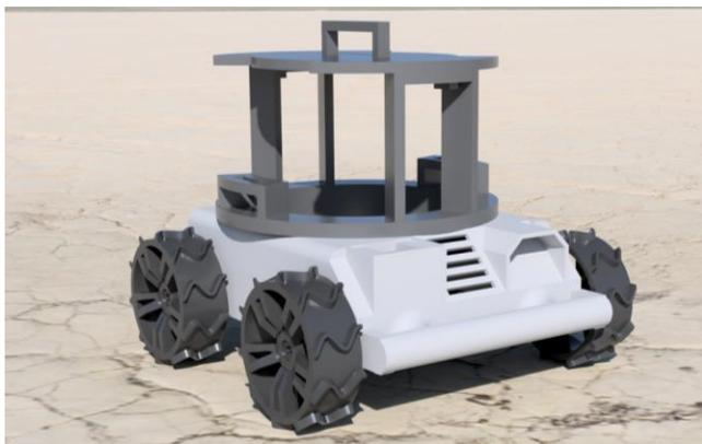
**Figure 2:** Rigid Chassis UGV
