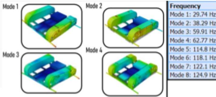
Figure 18: Vibration Modes with Constrained Center
