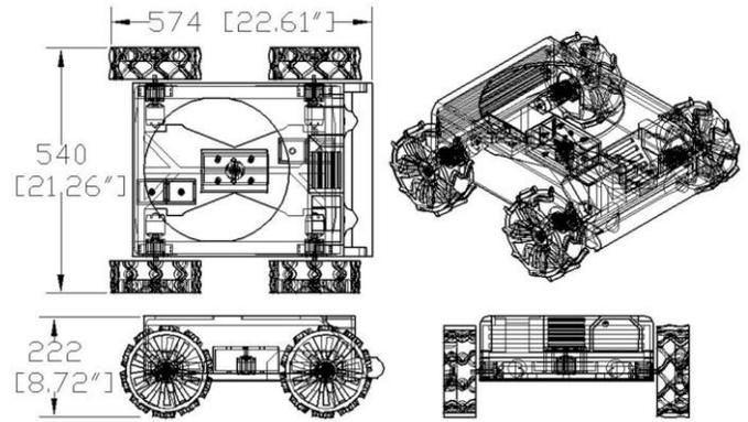
**Figure 13:** Rigid UGV Schematics
