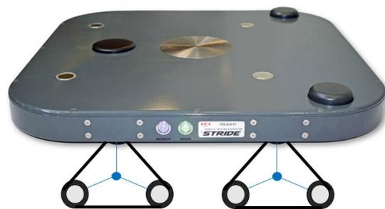
Figure 15: High-drive Track Design Concept
