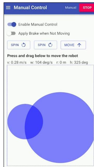
Figure 10: Robot GUI – Manual Control
