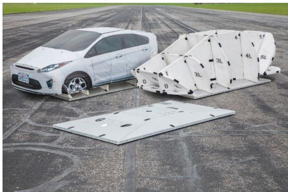
**Figure 1:** Guided Soft Target with Soft Car 360 Foam Car [1]
