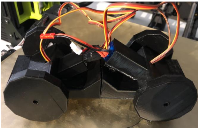
Figure 7: 4-wheeled vehicle in closed position after breaking away from build plate
