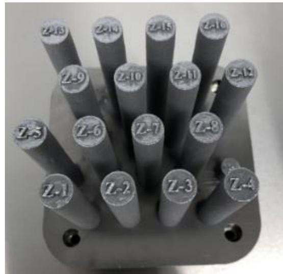
**Figure 2:** Tensile specimens printed from ATI Titan 23™ in SLM 125HL
