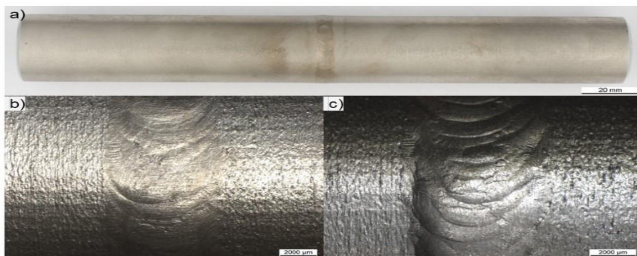
Figure 3. Two pipes TIG-welded together (a), Light microscopy photo (10x) of a weld seam of non-heat treated (b) and heat-treated IN718 (c).
