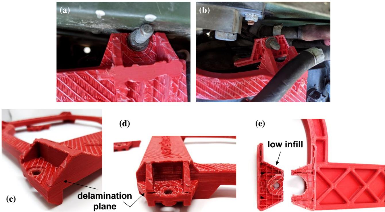
**Figure 2:** (a,b) Failure of as-printed ABS bracket during M998 installation. (c, d) Delamination failure mode for as-printed bracket. (e) Low infill as a contributor to poor interlayer strength.
