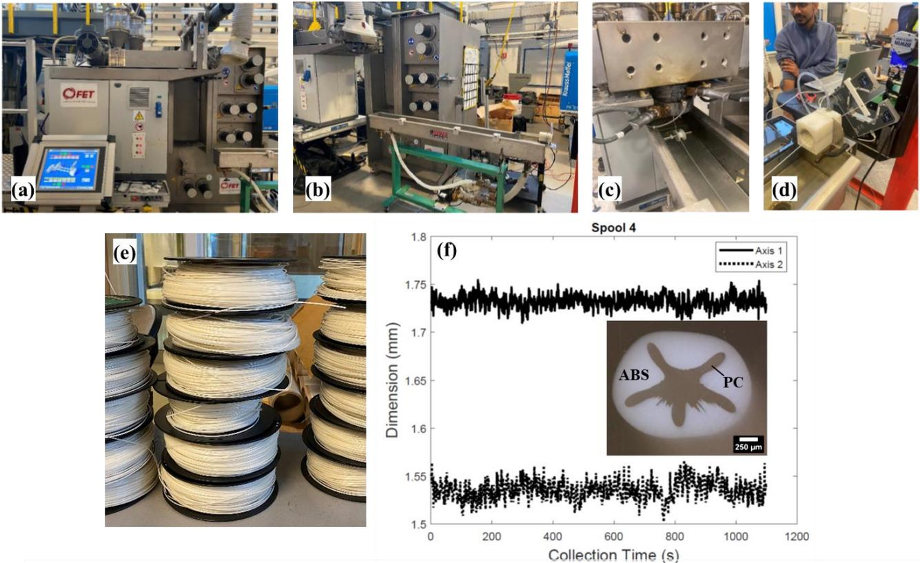
**Figure 6:** (a-d) Production of DM filament. DM filament (e) spools, (f) diameter data and cross-sectional micrograph.
