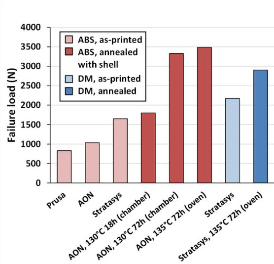
**Figure 5:** Quarter-section failure load for different print and annealing conditions.
