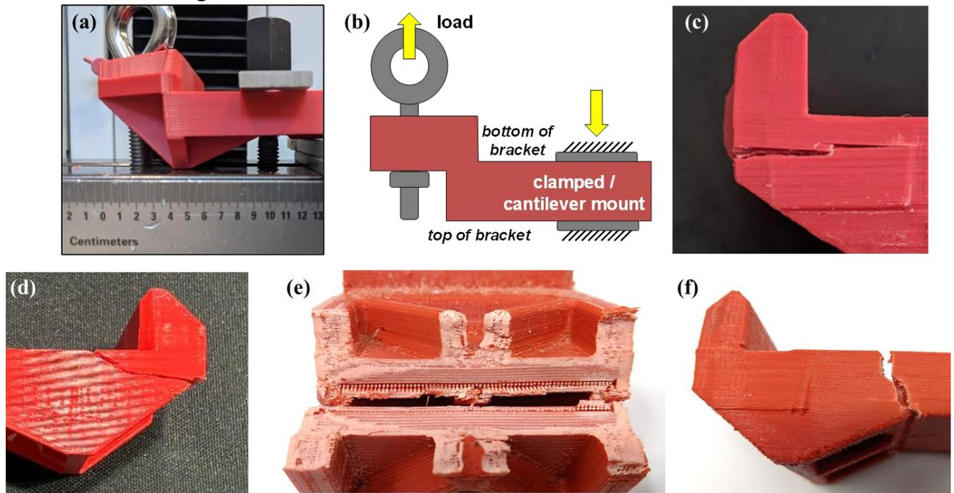
**Figure 4:** (a,b) Photo and schematic of load frame testing of quarter section. (a) As-printed AON3D and (b) as-printed Strataysys, and (e, f) annealed AON3D specimens after failure. The as-printed samples show significant delamination, whereas the annealed samples fail through layers.
