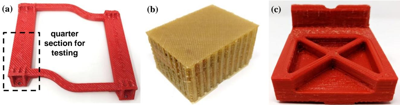
**Figure 3:** (a) Quarter section area used for load frame testing. (b) ABS quarter section printed in a dissolvable support shell (amber colored material). (c) ABS quarter section after annealing and support shell removal.
