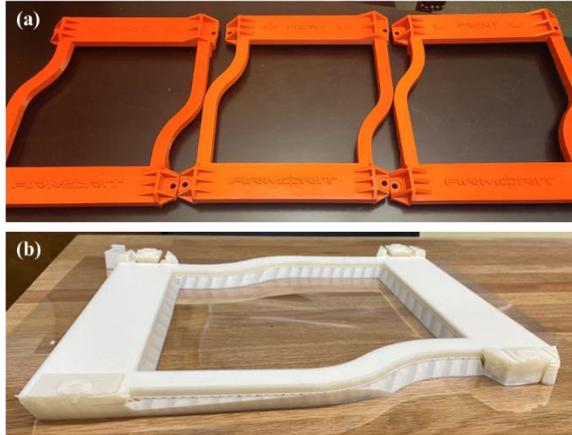
**Figure 8:** Full battery brackets printed using (a) ABS and (b) DM filament. The DM part failed mid-print, but is being re-printed for evaluation.
