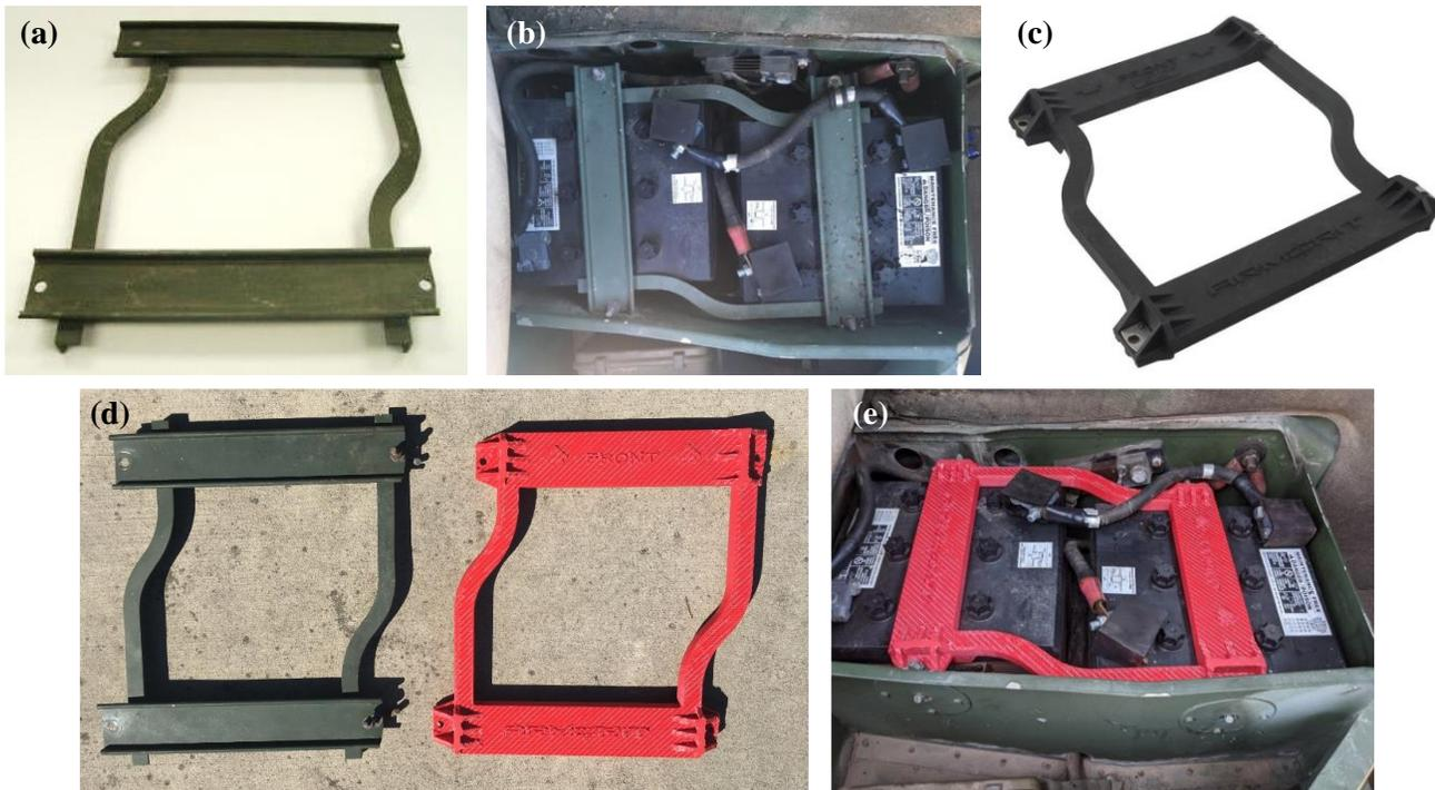
**Figure 1:** (a) Standard aluminum battery bracket, and (b) installed bracket on M998. (c) Aftermarket injection-molded polypropylene bracket. (d) Comparison of standard bracket and 3D printed bracket, and (e) 3D printed bracket installed on M998.
