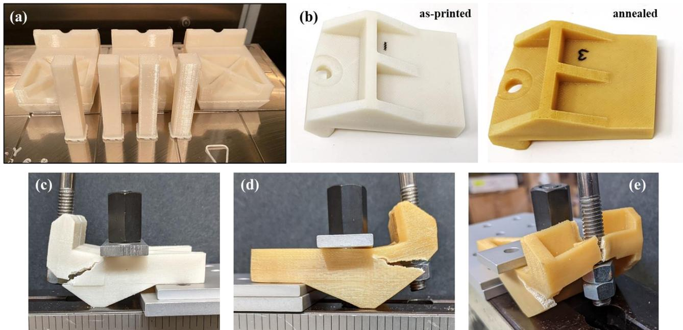
**Figure 7:** (a) Printed DM test specimens. (b) DM specimens after and before annealing. Images at failure for (a) as-printed and (b, c) annealed DM specimens.
