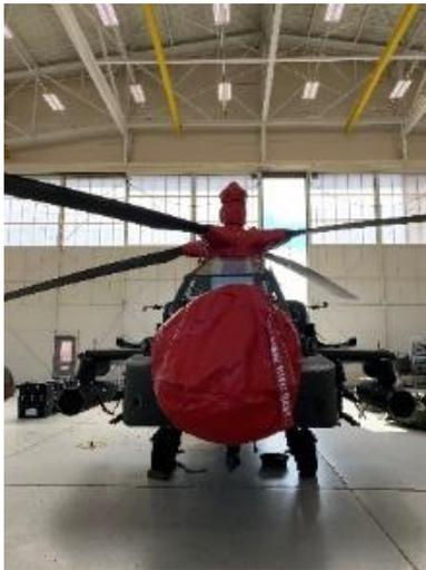
**Figure 17:** An ArmorDillo cover protecting an Apache rotor and M-TADS from corrosion and FOD.
