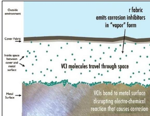
Figure 5: VCI migrating and bonding to the metal.
