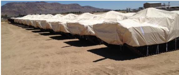
**Figure 1:** M1A1 tanks protected by a tan XT cover.
