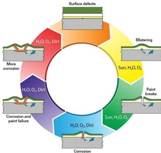
**Figure 4:** Paint failure and corrosion cycle.
