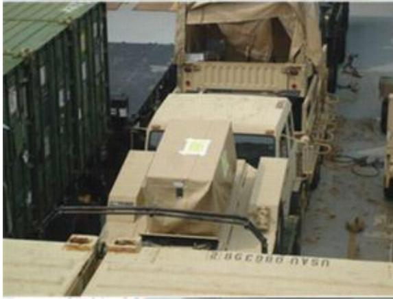
**Figure 5:** U.S. Army MEP-1040, 10kW 50/60Hz Generator protected by an ArmorDillo cover
