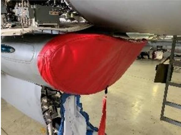
**Figure 16:** An ArmorDillo cover protecting an F-16's engine inlet from FOD.
