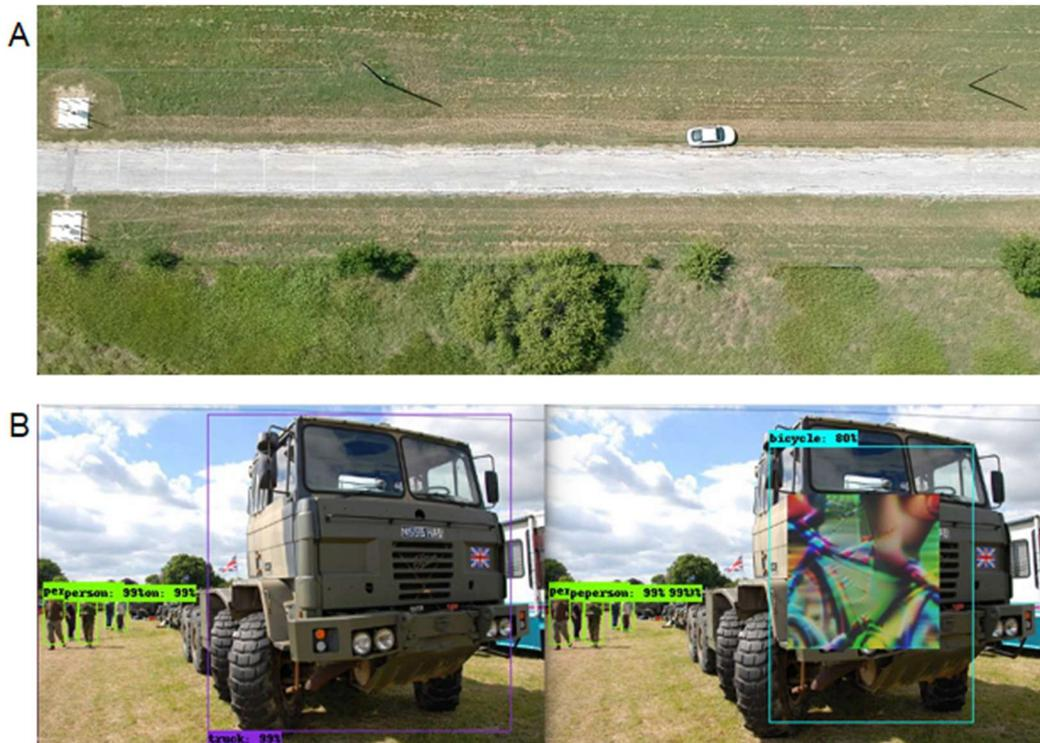
**Figure 1.** Examples of sensor manipulation include A) An offset applied mid-route forces an automated vehicle off the road, and B) an object classification algorithm classified as a truck as a bicycle
