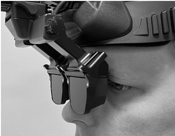
Figure 1. An SA-62 HMD system in a laboratory at the Georgia Tech Research Institute (GTRI).
