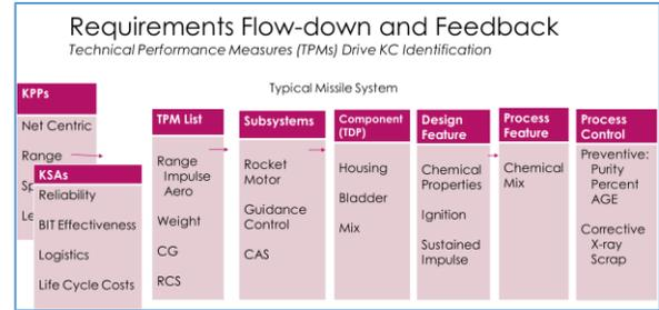
Figure 11, **Block and Performance Diagrams** can help define the relationships between subsystem elements and functional product design characteristics of interest to help interrogate the manufacturing risk and establish relevant control as needed.
