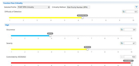
Figure 7: Criticality Model associates qualitative parameters with failure concepts defined in the MADE failure diagram.
