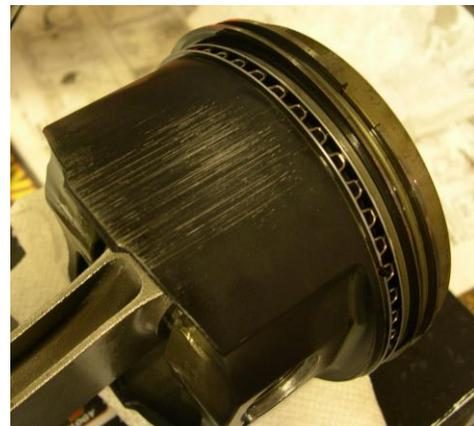
**Figure 5C:** AAPC protected this piston from ingested sand, and was used to restore the surface and resize the skirt for the newly honed bore dimension during overhaul.
