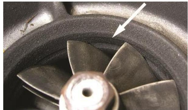
**Figure 9:** Rotor bedded into soft coating - perfect seal (zero clearance and zero friction) after 150,000 miles
