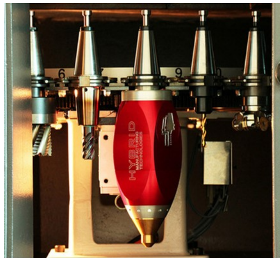
Photo courtesy of Hybrid Manufacturing Technologies Figure 1: Typical DED AM print head among a series of cutting tools.
