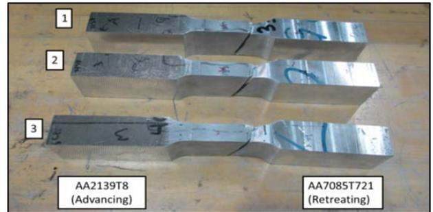
Figure 4: A2139-T8 to AA7085-T721 tensile test result.
