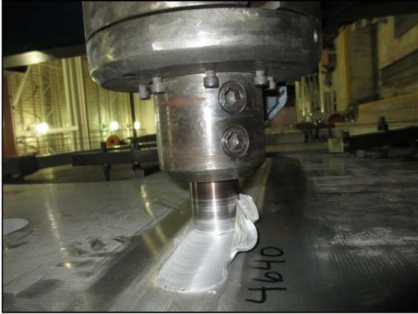
Figure 2: Friction stir welding process.
