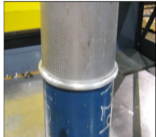
Figure 3: Finished large diameter/heavy wall aluminum to steel inertia weld. Part has a 127-mm diameter and 10-mm wall.
