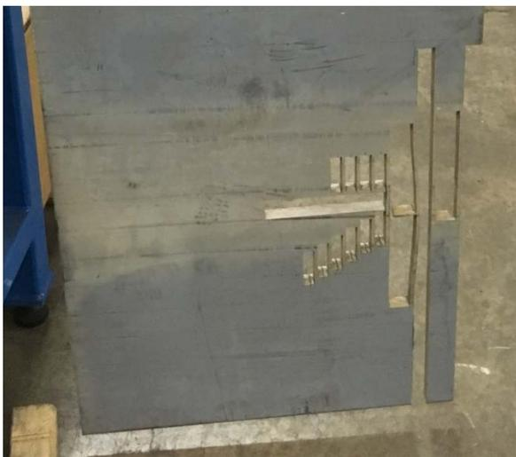
Figure 19: Armor plate after removal of test coupons
