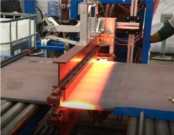
Figure 28: Plate being heated locally prior to forming
