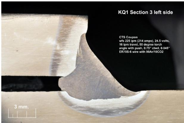
Figure 36: Macro section through a CTS weld showing the pre-machined root notch
