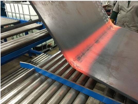
Figure 29: Plate immediately after forming
