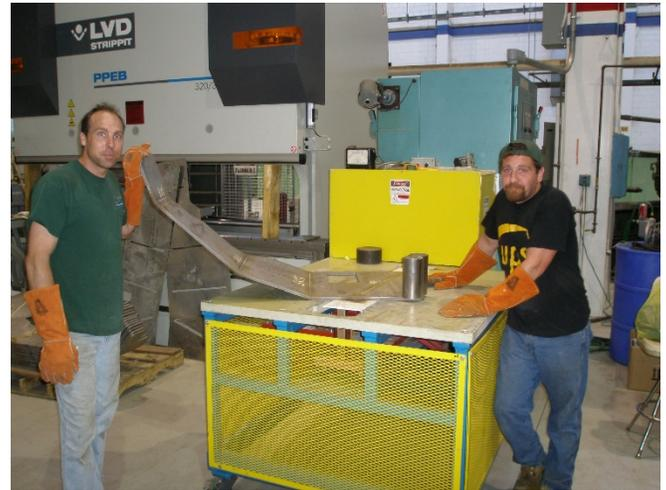
Figure 3: Single sided induction table and 3 bend part
