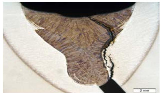
Figure 39: Multiple cracks in Tekken test
