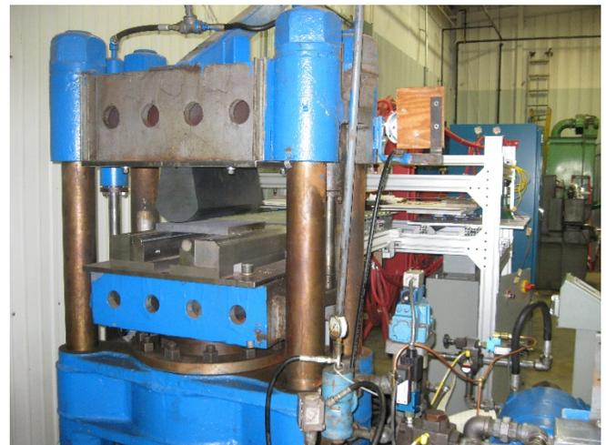
Figure 6: Hydraulic press and oscillating induction station
