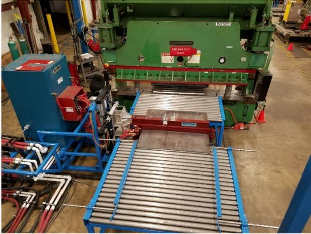
Figure 16: 175 ton press brake and induction coils for 20 mm plate
