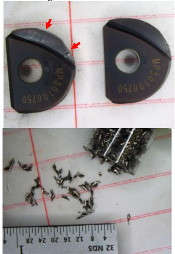
**Figure 22.** Stereoscopic images of (top) the cutting bits in the used (leftmost) and unused (center) bits, and the produced cutting swarf (bottom)
