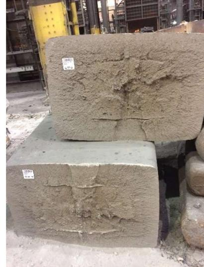
**Figure 4:** Fracture surface of a 34”x47” ingot that failed during solidification and cooling.
