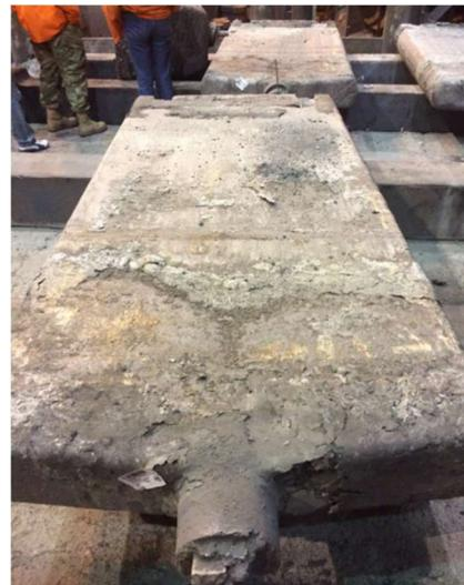
**Figure 2:** As-cast ingot of FeMnAl steel produced with high silica teeming flux
