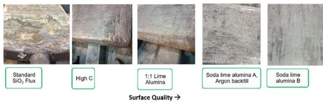
**Figure 3:** As-cast ingot surfaces resulting from a variety of fluxes used, with improving surface quality from left to right in the figure.
