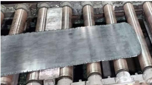
**Figure 6:** Forged billet rolled to 0.5" thick plate at a soaking temperature of 2128°F. Plate is ~ 6' wide.
