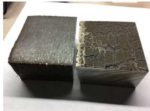
**Figure 7.** Comparison of surface quality of (left) forged and rolled at 2150°F, and (right) rolled at 1950°F plate from the same pour
