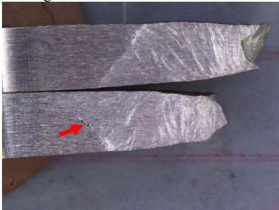
**Figure 18.** Tensile specimen post-testing showing small tear at the interface between the fusion zone and base metal.
