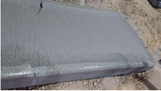
**Figure 5:** Ingot after rolling attempt at 1950°F showing substantial transverse tearing after minimal reduction
