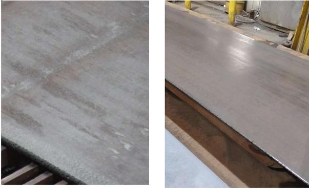
**Figure 8.** Plate rolled at 2200F from (left) forged billet and (right) as-cast ingot, showing overall surface quality and edge cracking
