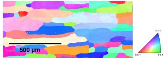
**Figure 3:** EBSD orientation map of the HAZ in the transverse cross section.
