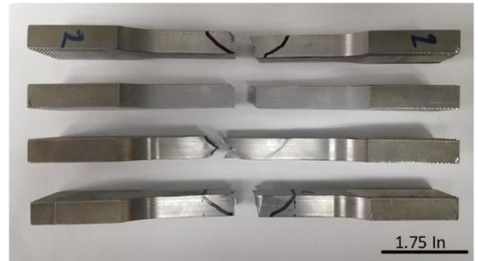
Figure 12 Cross weld tensile specimens after failure.
