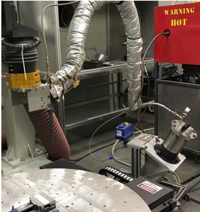
Figure 2: VRC Gen III™ cold spray setup
