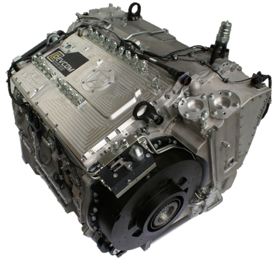
Figure 4. The Advanced Combat Transmission (ACT)
