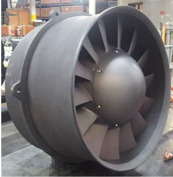
Figure 11. The high-voltage electrical fan
