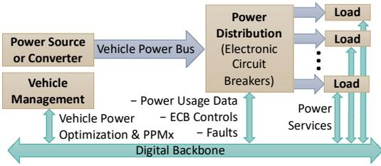
**Figure 3:** Vehicle power architecture enhancements made possible using intelligent ECB subsystems.
