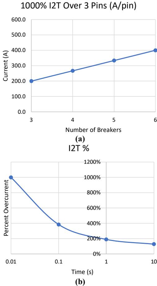
**Figure 6:** (a) Maximum overcurrent per pin when allocating three pins for module input. (b) Example I<sup>2</sup>T curve overcurrent as a percentage of specified max ECB steady-state current.
