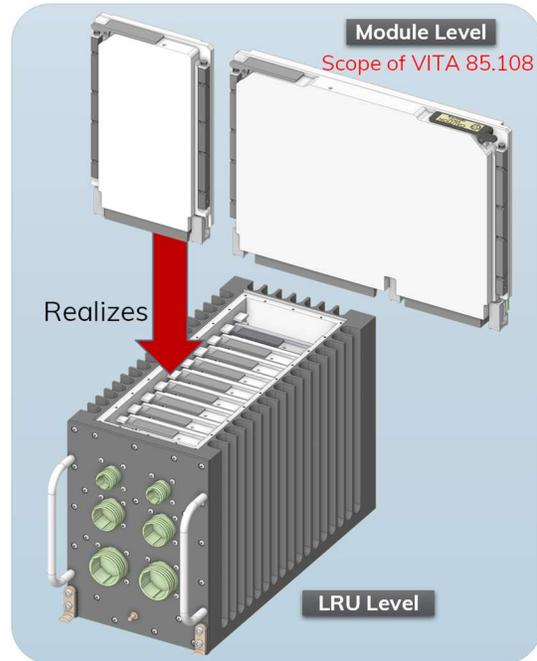
**Figure 4:** At the module level, the utilization of VPX 3U and 6U definitions help to realize an LRU supporting providing power distribution functionality.
