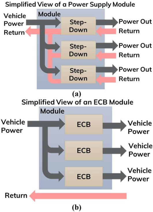
**Figure 2:** Functional differences between (a) typical power supply module and (b) an ECB module indicating the need for a distinct standard.
