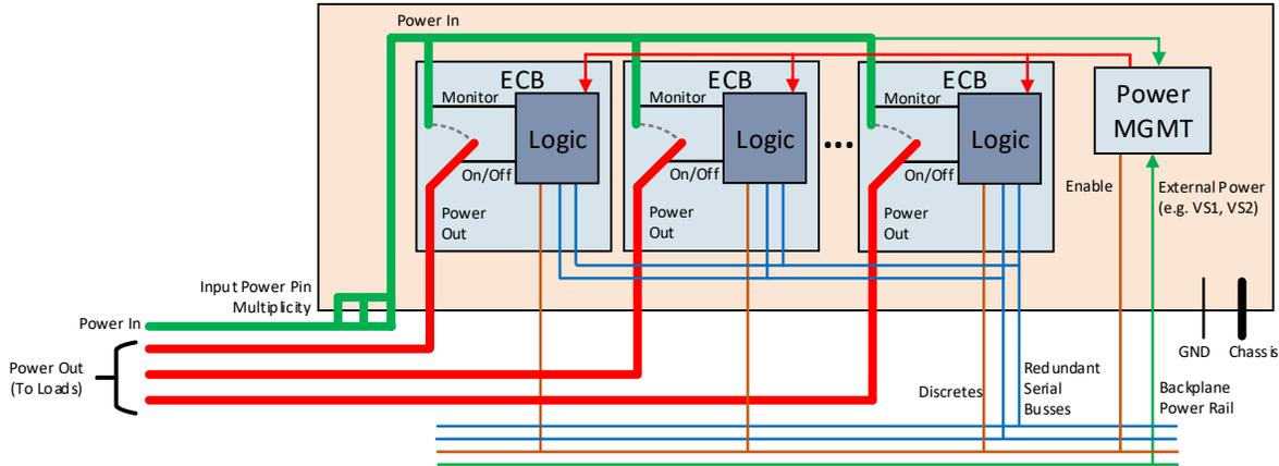
**Figure 5:** ECB module architecture incorporating the interfaces necessary to meet functional needs of intelligent power management.
