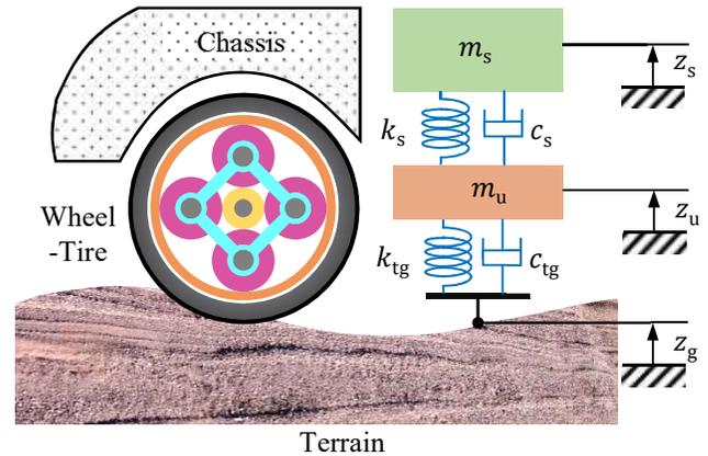
**Figure 2.** The sprung-unsprung mass system of the SWM.
