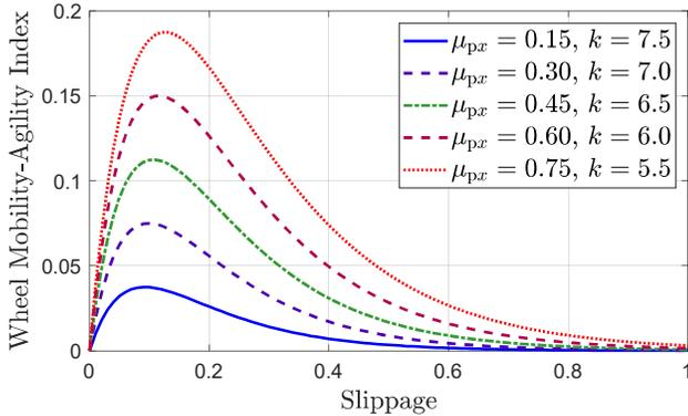
**Figure 7.** Illustration of the WMAI for different friction coefficient attributes based on the WMI.
