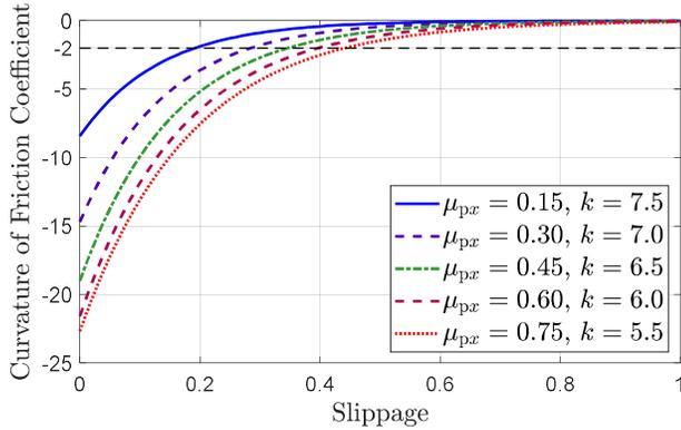
**Figure 5.** The curvature of the friction coefficient as an indicator of the slippage behavior.
