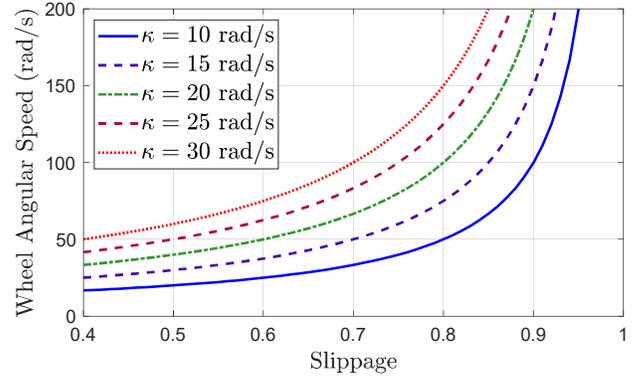
**Figure 4.** The effect of the slippage growth on the wheel angular speed at the mobility critical condition.
