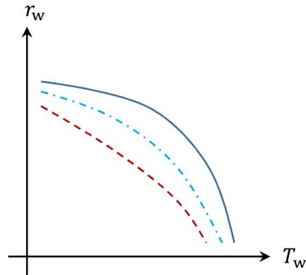
**Figure 6.** The general nonlinear relation between the instantaneous tire rolling radius and the wheel torque.
