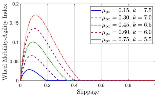
**Figure 8.** Illustration of the WMAI for different friction coefficient attributes based on the modified WMI.
