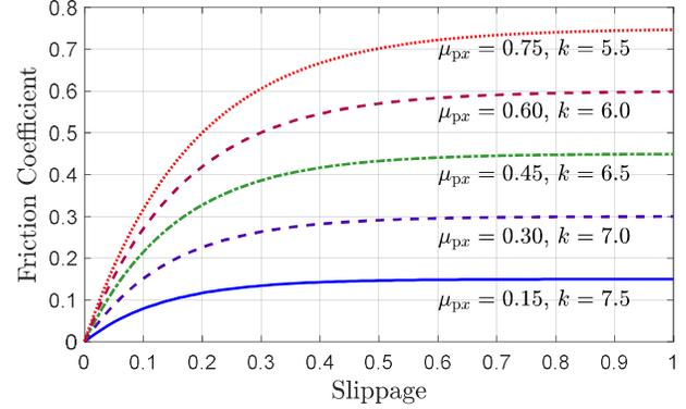
**Figure 3.** The typical relation between the friction coefficient and the slippage in off-road terrains.
