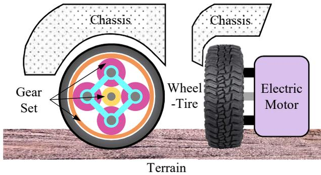
**Figure 1.** The propulsion system of the SWM.
