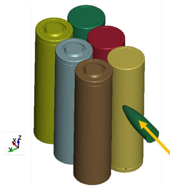
**Figure 1:** Geometry of the 3P2S configuration of 18650 cells used in this study and direction of loading under ultra-high strain-rates
