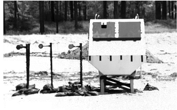
Figure 25a: Test setup with AGH for free air detonations [33]
