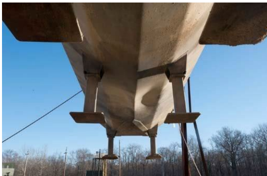
Figure 6: Deformed underside of AGH
