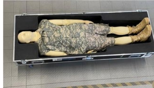
Figure 29: PRIMUS dummy used in live fire test using the AGH [38]
